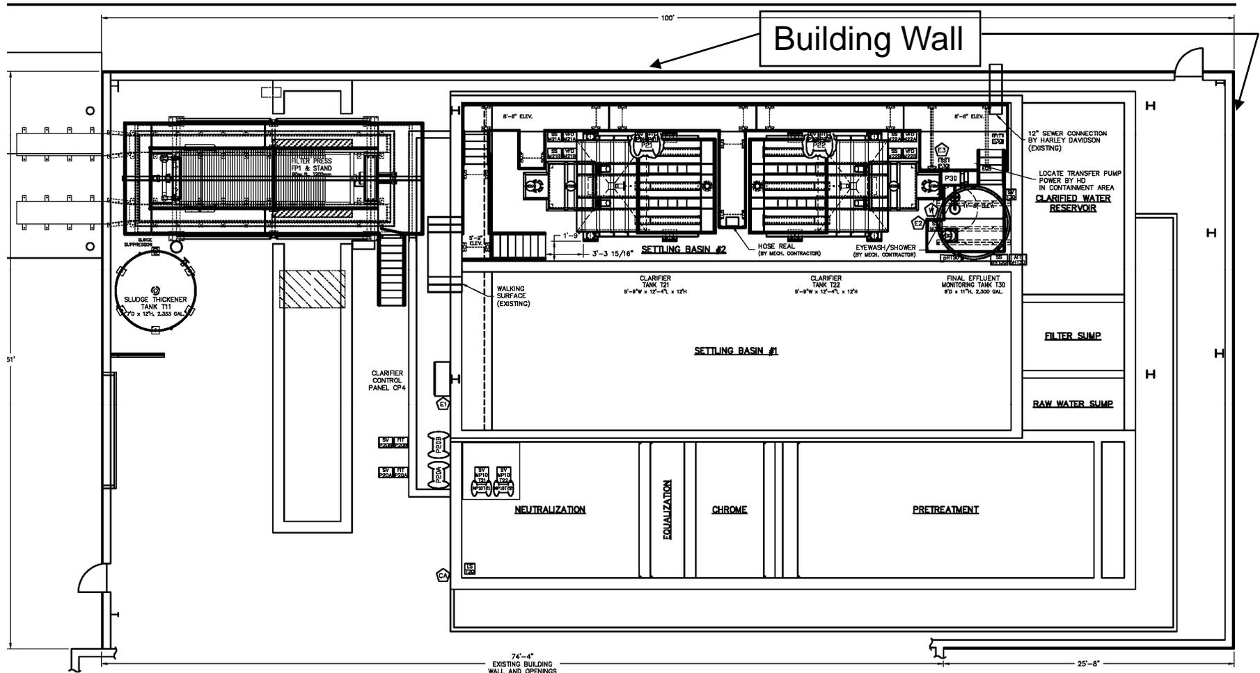
**Figure 4** – June 20, 2007 proposed (existing) layout [J. Mark Systems] showing Bldg 41 wastewater tank area only. Note proposed use of northern settling basin with a new lamella clarifier; new location of sludge filter press (indoors); and existing sludge pit (west of settling basins). Building walls and current roof over the WWTP basins was constructed circa 1980, according to other available construction drawings.
